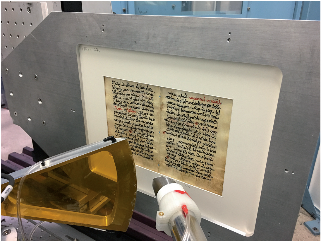
Fig. 5: SGP bifolio mounted on translation stage in SLAC SSRL beamline hutch (© R.B. Toth Associates)
